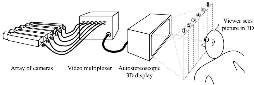
Figure 1: an autostereoscopic camera system. The six views captured by the six cameras are multiplexed onto the autostereoscopic display, allowing the viewer to see the scene in three dimensions.
