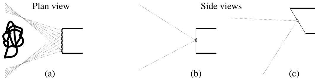
Figure 3: (a) the autostereoscopic laparoscope will be capable of a field of view of  $60^\circ$ . It will be possible to design it so as to view either straight ahead (b) or at, for example,  $30^\circ$  (c).
