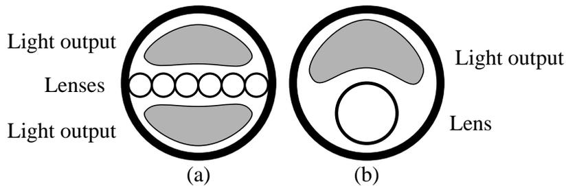
Figure 2: (a) the distal end of the autostereoscopic laparoscope, compared with (b) the distal end of a conventional 2D laparoscope.
