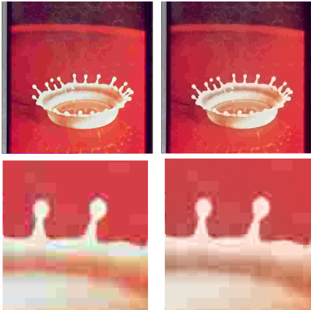
Fig. 14. Joint bilateral filter example. Left: JPEG compression using 2 \times 2 chrominance subsampling and IJG quality factor 10, file size 8,053 bytes. Right: JB-JPEG compression using 5 \times 5 chrominance subsampling, IJG quality factors of 11 for luminance and 75 for chrominance, file size 7,822 bytes. As in Figure 13, joint bilateral filtering has prevented the colour shifts that are visible in the JPEG compressed image. The enlarged portion of the images shows that the JPEG compression has introduced noticeable and disturbing colour shift artefacts. Note, however, the large area of constant colour in the main image: this exhibits typically JPEG blocky artefacts in both images. These artefacts are present in the luminance channel and thus the JB-JPEG algorithm does not remove them.
