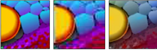
Fig. 2. Examples at high levels of compression. Left: original. Centre: JPEG compression artefacts. Right: “compression by colorization” artefacts: the JPEG artefacts have practically vanished but there is some loss of vividness.
