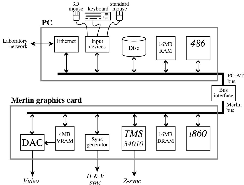
Figure 5: The architecture of the current computer system used to drive the display. The host PC acts as a server for access to disk, input devices, and the network. The i860 on the graphics card is the main processor and performs all of the rendering. The TMS 34010 generates the Z-sync and ensures that the correct field is being output by the DAC at all times. The Merlin graphics card was bought off-the-shelf, but any suitably flexible graphics system could be used to drive the display.
