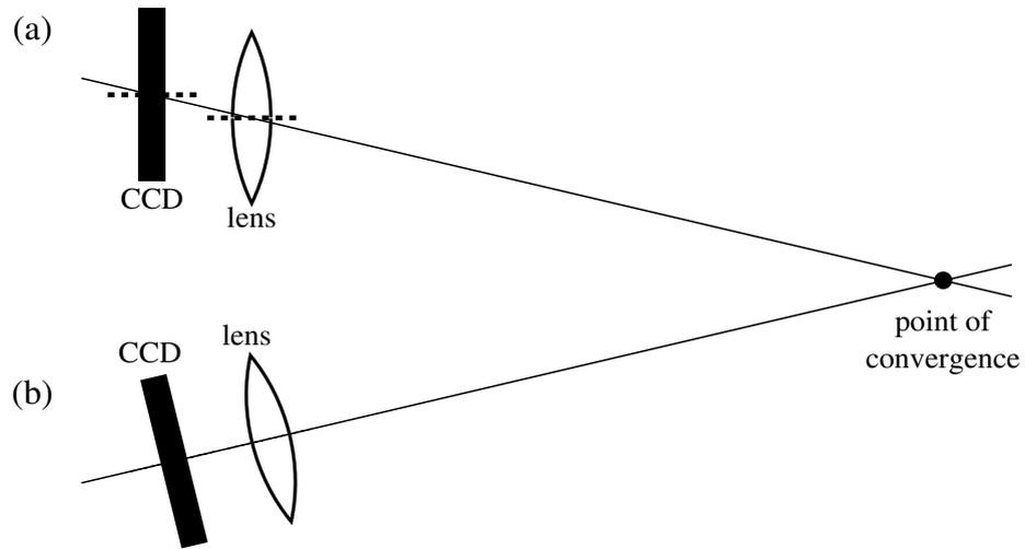
**Figure 5.** (a) an off-axis setting of the camera lens can be used instead of the inefficient arrangement shown in Figure 4. Compare this with (b), the radial arrangement, where a standard camera can be used with no modification and with no loss of part of the CCD.
