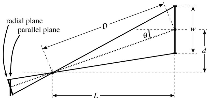
**Figure 8.** The geometry for a single camera showing the important parameters. Assuming a pinhole camera, the same light rays hit the radial plane as hit the parallel plane; they are merely sampled differently. Note that the geometry to the left of the pinhole is congruent to that on the right.
