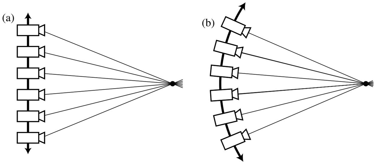
**Figure 1.** (a) the parallel configuration; (b) the radial configuration.
