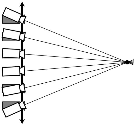
**Figure 6.** Cameras are arranged as for the parallel case (Figure 1(a)). Each is rotated about the appropriate principal point of its lens system so that their axes all pass through the point of convergence.
