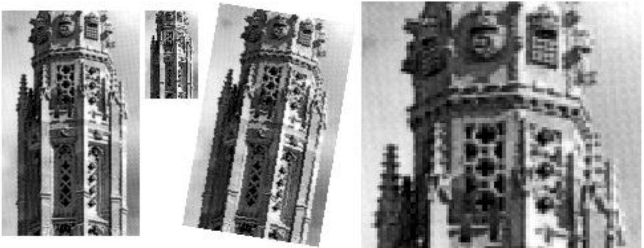
**Figure 11.** Examples of the artifacts which occur with nearest-neighbour reconstruction. At left is the original. At right, an enlarged version, clearly showing the block structure. In the middle are a reduced version, showing the problems of undersampling, and a rotated version, showing artifacts along the vertical edges of the tower.
