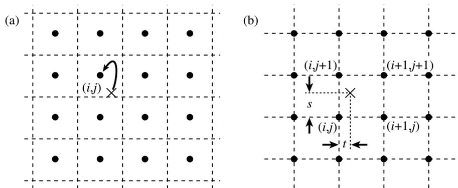
**Figure 13.** (a) nearest-neighbour reconstruction takes the nearest sample value to the transformed sample point while, (b), linear reconstruction takes a weighted mean of the four nearest sample points  $F'(x, y) = (1 - t)(1 - s)F_{i,j} + (1 - t)sF_{i,j+1} + t(1 - s)F_{i+1,j} + tsF_{i+1,j+1}$ .
