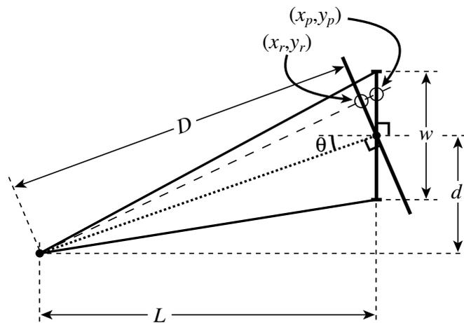
**Figure 9.** The geometry used in this analysis. Both radial and parallel planes pass through the point of convergence. A ray from the pinhole intersects the radial plane at  $(x_r, y_r)$  and the parallel plane at  $(x_p, y_p)$ . These are coordinate systems local to each plane. The origins of both these coordinate systems are at the point of convergence, with the  $y$ -axes perpendicular to the plane in which lie the point of convergence and the cameras' principal points.
