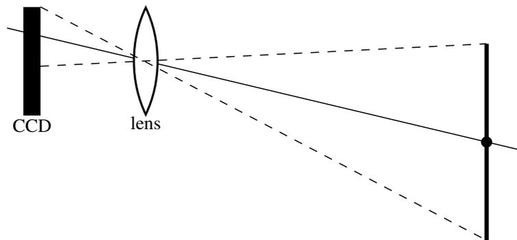
**Figure 4.** When capturing images in the parallel configuration with conventional cameras, only part of the CCD images the desired scene. The resulting image needs to be clipped to ensure that only the appropriate part is used.
