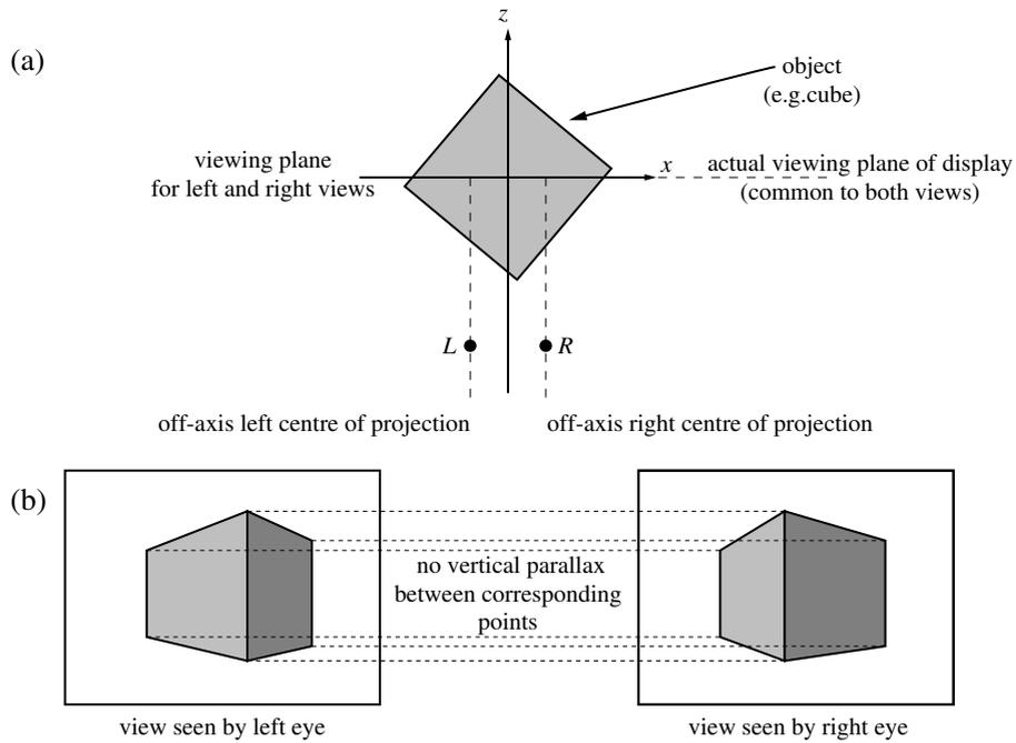
**Figure 3.** Parallel configuration: (a) the geometry of parallel capture of perspective views for stereo; (b) correct stereo image resulting from parallel capture of perspective views.
