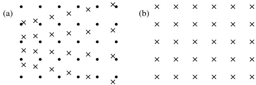
**Figure 10.** The circles represent sample points in (a), the original image, while the crosses represent sample points in (b), the resampled image. Each sample point in (b) is transformed to its equivalent location in (a) and the original sample points in the immediate vicinity are used to generate the resampled value.
