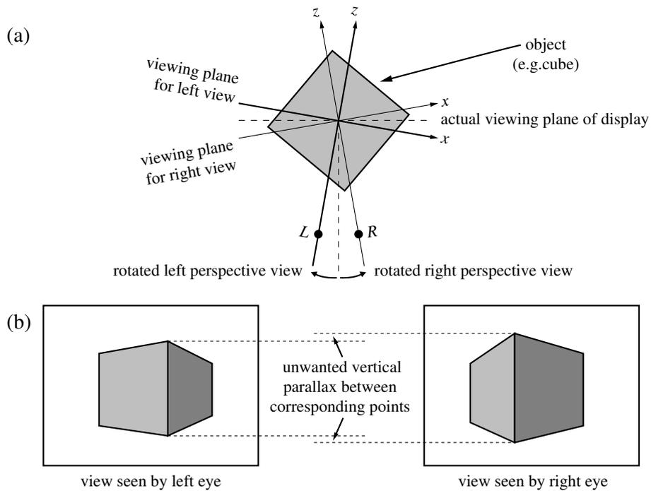
**Figure 2.** Radial configuration: (a) the geometry of rotation of perspective views for stereo; (b) distortions in the stereo image due to rotation of the perspective views. These distortions are caused by displaying both rotated views on the display's unrotated viewing plane.
