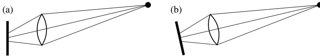
**Figure 14.** The image of an out of focus point formed in (a) the parallel case and (b) the radial case.
