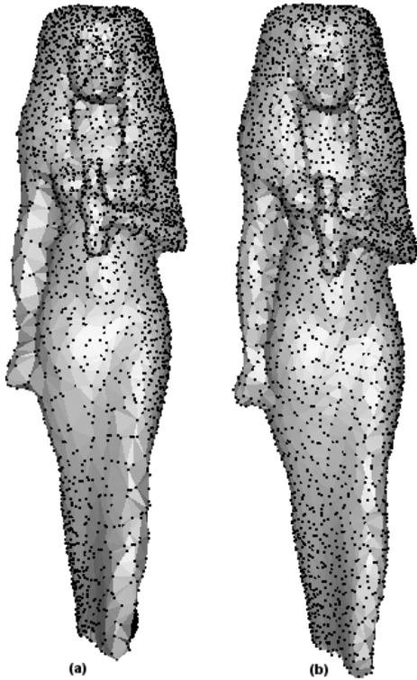
Figure 4. Feature-sensitively distributed point sets generated by adaptive simplification using local curvature estimation over rendering of corresponding mesh reconstructions. (a)  $\rho = 8.00$  (b)  $\rho = 5.50$ .
