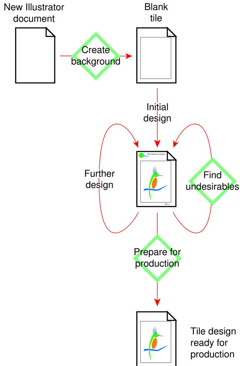
Figure 2: The position of the three proposed plug-in filters in the design cycle. One is used to create a blank tile, one is used during the design process to find undesirable features, and the third is used to remove extraneous information from the file and perform a final check on the design before the tile is sent into production.
