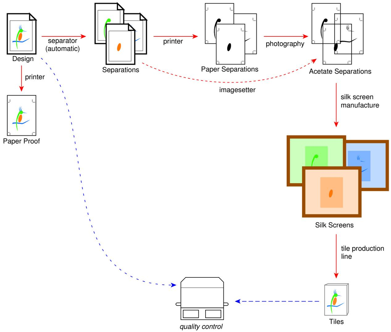
Figure 1: The stages involved in taking a finished (valid) tile design to production.
